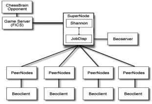
Fig 1: Simplified schematic of the ChessBrain architecture.
